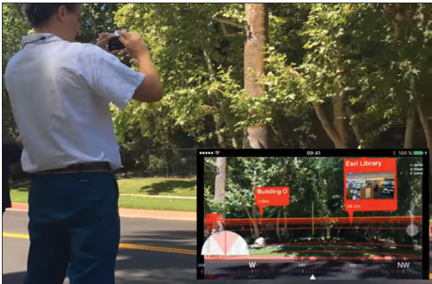
Esri AuGeo displays facility information on top of the user’s live camera view. The inset picture in the lower right corner is what users see on their phones.
